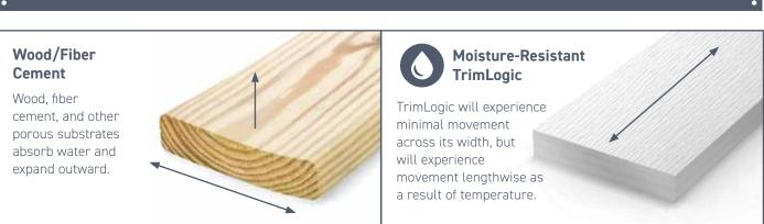
Understanding the unique expansion and contraction properties of different building materials is crucial for successful installations. TrimLogic, a new PVC trim product, has distinct installation requirements compared to wood or fiber cement. Adhering to these specific TrimLogic guidelines is essential for optimal performance and to maintain your warranty.
